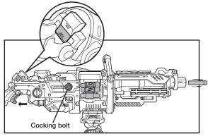
NOTE: If you see a white piston sticking out behind where the belt sits on the gear, pull the cocking bolt back slightly until the piston retracts.
